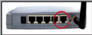
INTERNET or WAN Port on the Router
